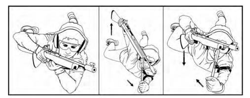
Figure 7 Pumping the air rifle
